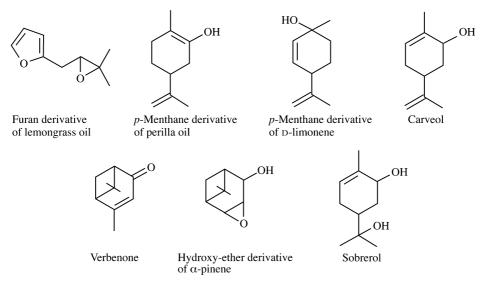
Figure 2. Chemical structures of air-oxidation products.
