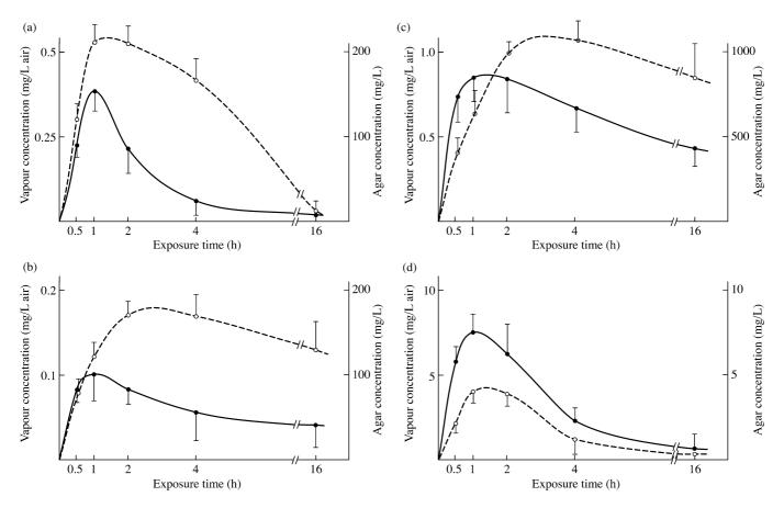
**Figure 1.** Time courses of vapour and MHA concentrations of essential oils at MID against *S. pnuemoniae* at 37°C in an airtight box. Concentration was expressed by average  $\pm$  s.D. (n = 3). A solid line and a dotted line indicate vapour and agar concentrations, respectively. (a) Citral at 6.25 µg/mL air; (b) thymol at 3.13 µg/mL air; (c) terpinen-4-ol at 50 µg/mL air; (d) D-limonene at 200 µg/mL air.
